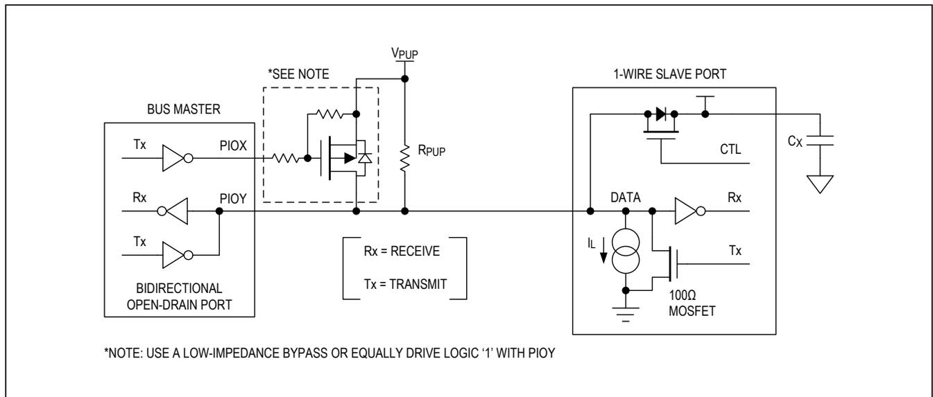
Figure 2. Hardware Configuration
