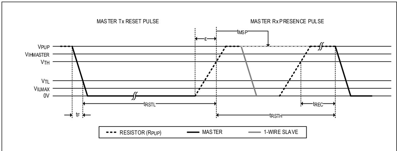
Figure 3. Initialization Procedure: Reset and Presence Pulse
