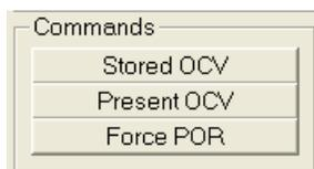
The Commands section provides access to the commands of the Command Register. Left-click on the Stored OCV button to force an OCV Calculation based on the voltage stored as the Initial Voltage. This will modify both the Relative Capacity Register and the Last OCV Register.
