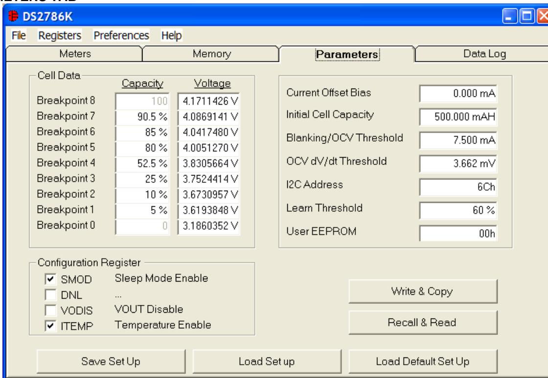
The Parameters Tab gives the user access to the entire Parameter EEPROM memory. The DS2786 comes preloaded with a best fit curve that was calculated based on characterization data taken from cells of various sizes and manufacturers. To change any of this information, simply click on the desired text field and enter the new value.
