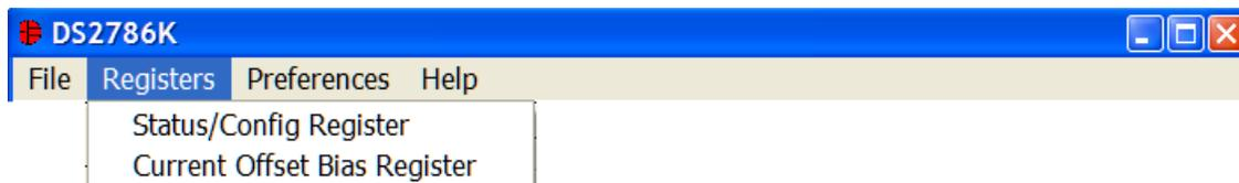
The Registers Menu gives immediate access to the Status register and the Current Offset Bias Register of the DS2786. Selecting either of the registers will open an individual control window giving the user a description of each register bit and the ability to read or write it.
