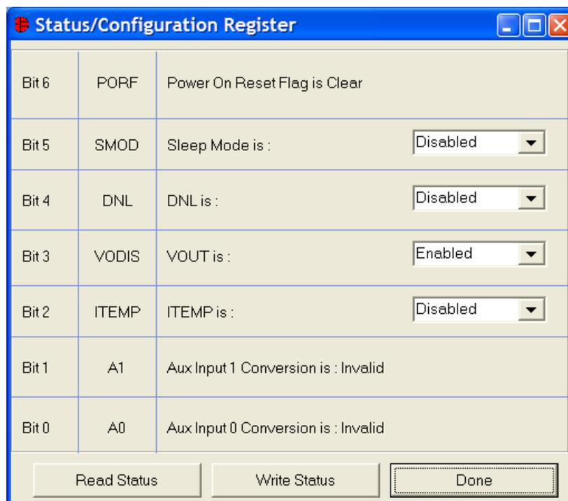
The present state of all register bits are displayed immediately upon opening the register window. R/W locations contain a selection field or command button to allow the user to determine their state. Pressing the Write Status button will write the new value to the register and read the corresponding register inside the DS2786 to verify the correct value was written. Note: This window does not copy these values to EEPROM. To copy the desired values to EEPROM, see the Parameters section.
