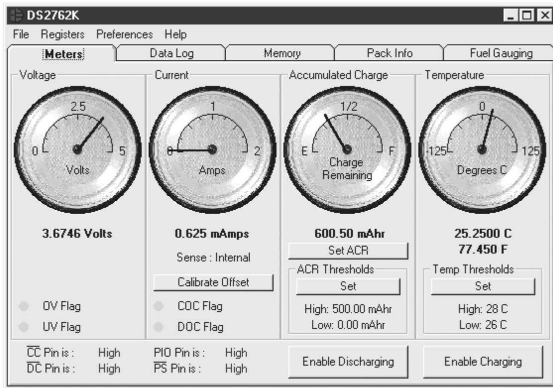
The user can bring up the Update Current Accumulator window by left clicking the Set ACR button. This window allows the user to enter values for the Current Accumulator Register and Rated Battery Capacity in mAH. Rated Battery Capacity is used to determine full-scale range on the Charge Remaining Meter only. It has no affect on device operation.
