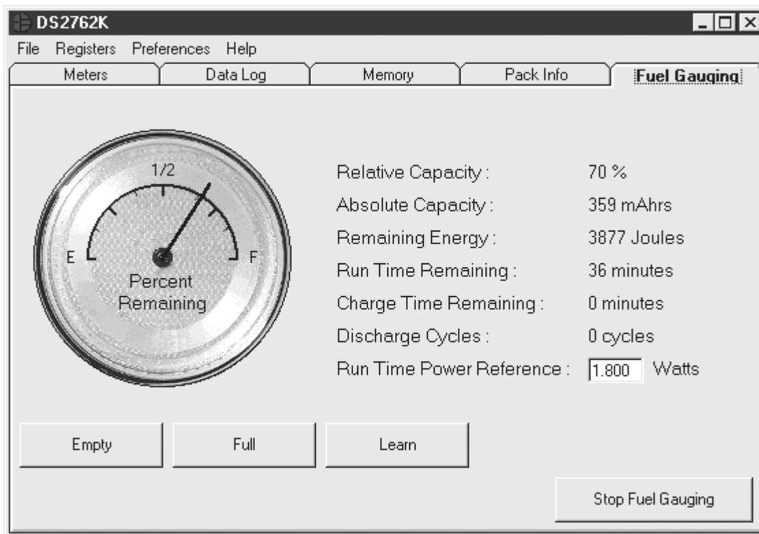
The remaining run time is calculated using the Run Time Power Reference input from the user. Instantaneous current measurements in the user's application can vary greatly. By using a reference scalar instead of actual current and voltage measurements, the program produces a stable estimation of remaining run time. The user should enter the largest expected power draw from the device into the Run Time Power Reference field for the most accurate estimation.
