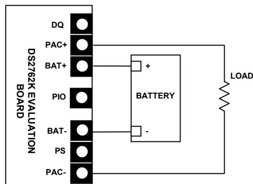
Figure 2b. Discharging Circuit
