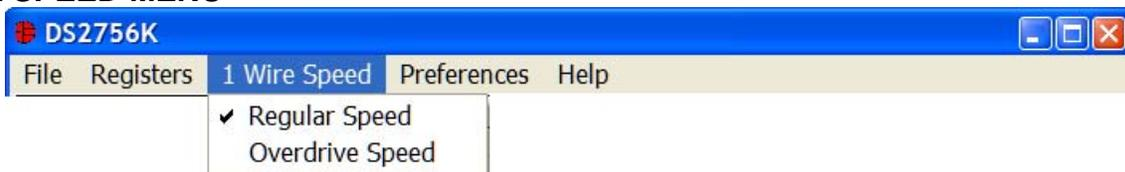
The 1 Wire Speed Menu allows the user to select the appropriate 1 Wire timing. The speed the device uses is determined by the state of the OVD bit in the Status Register.
