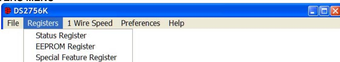
The Registers Menu gives immediate access to all three status and function registers of the DS2756. Selecting any of the registers will open an individual control window giving the user a description of each register bit and the ability to read or write it. See the status register window example.
