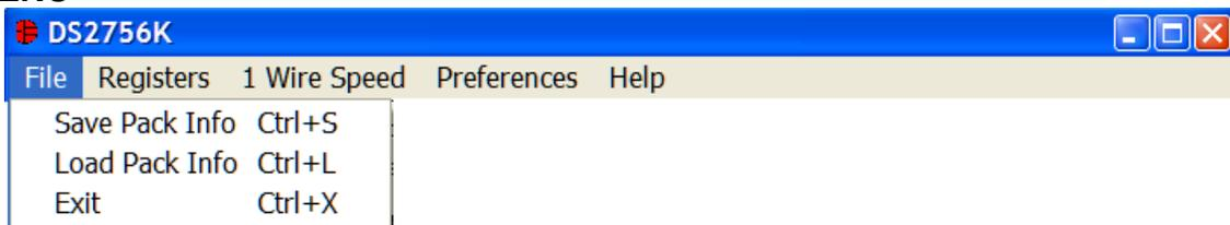
The File Menu allows the user to store information from a file directly into the Device Setup, Battery Data, and Fuel Gauging Data sections under the Pack Info Tab or take the same Pack Information and store to a file. These functions do not directly write or read the DS2756. It is still necessary for the user to store or recall this information to or from the device by issuing a WRITE or READ command under the Pack Info Tab.
