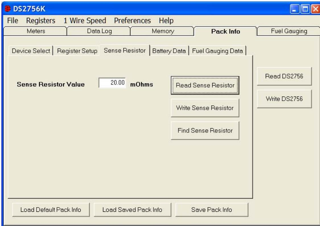
The Sense Resistor Select sub-tab allows the user to correct the current measurements if a different value of sense resistor is used. All DS2756s with an integrated sense resistor use 20mΩs. If the sense resistor is located externally, the user should select the external resistor radio button on this tab, then enter the value of the resistor in mΩs in the Sense Resistor Value field and then click the WRITE SENSE RESISTOR button.
