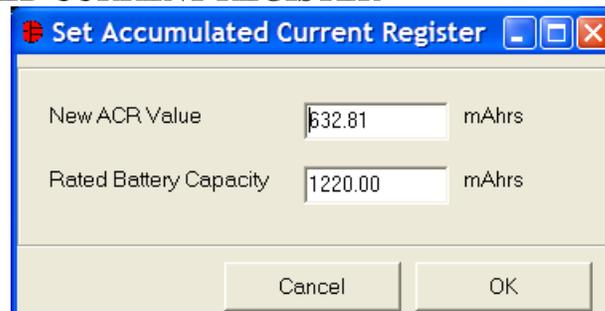
The user can bring up the Set Accumulated Current Register window by left clicking the Set ACR button of the Meters Tab. This window allows the user to enter values for the Accumulated Current Register and
