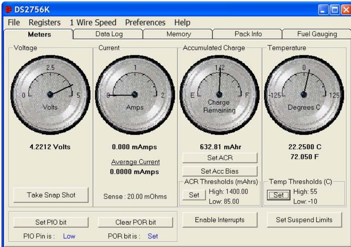
The Meters Screen displays the latest real-time measurements of cell voltage, temperature, current and accumulated charge with both analog meter readouts and digital values. The sense resistor value used to calculate the current reading is shown in the current section. Left click on it or go to the sense resistor sub-tab under Pack Info to change this value.
