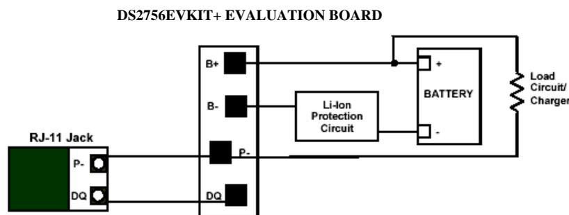
Figure 1: PD010203 Cell, Load, and Charger Connections
