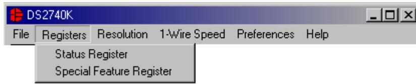
The *Registers Menu* gives immediate access to the *Status* and *Special Feature Registers* in the DS2740. Selecting one of the registers will open an individual control window giving the user a description of each register bit and the ability to read or write it. See the Status register window example in the next section. The individual control window can also be displayed by left clicking on any label referring to any of the bits of the *Status* or *Special Feature Registers*.
