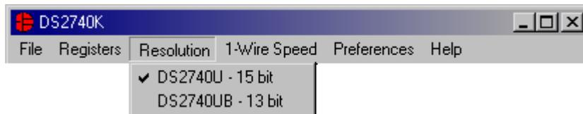
The *Resolution Menu* allows the user to select which version of the DS2740 is being used. This selection will affect the value of the units used to calculate the current. The software cannot detect which version of the DS2740 is being used, so if the wrong version is selected, the current reading will be off by a factor of 4.
