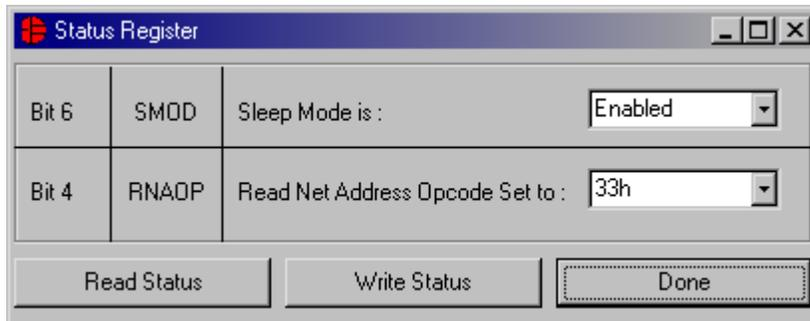
The present states of all register bits are displayed immediately upon opening the register window. Read/write locations contain a selection field to allow the user to determine their state.
