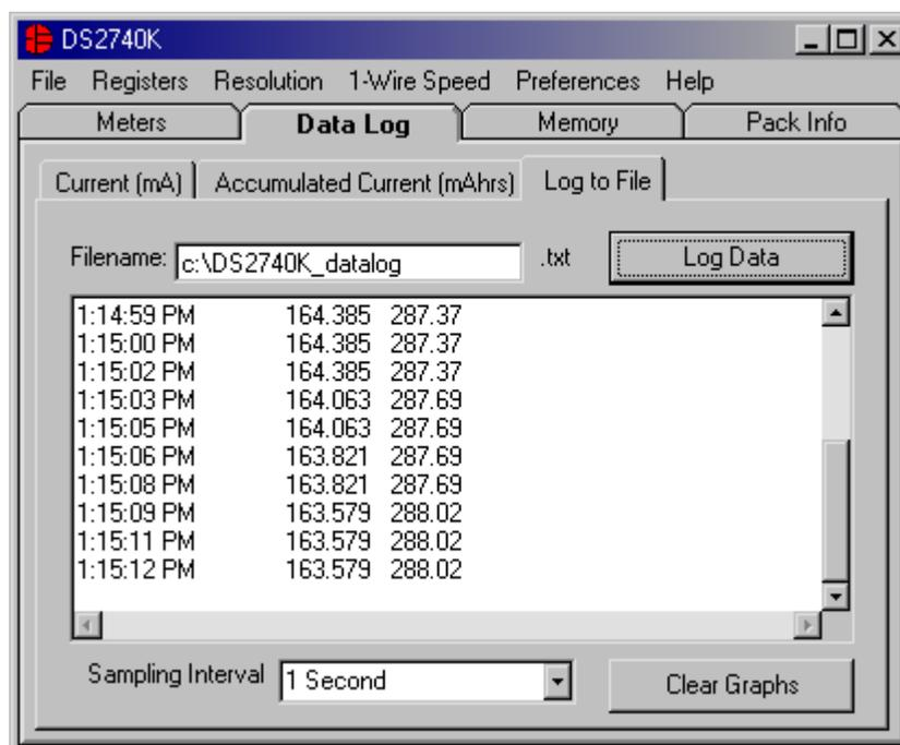
The *Log to File* sub-tab contains control information for storing all log data to an ASCII file. The default filename is c:\DS2740K\_datalog.txt, but can be modified in the filename text field. The *Log Data* button toggles data logging off and on. Data will be stored at the same interval selected for updating the graphs in the tab-delimited format of:
