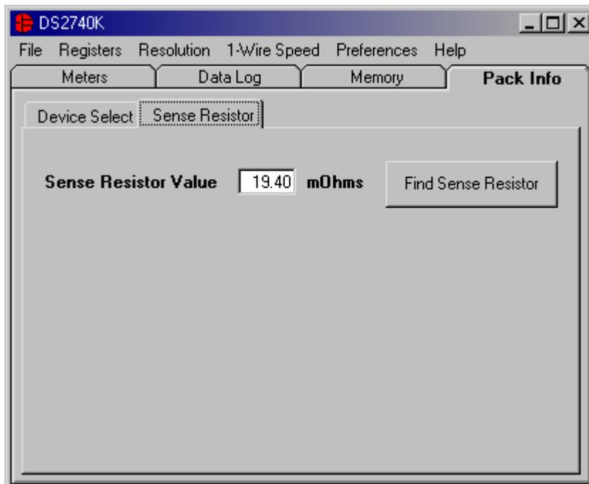
The *Sense Resistor* sub-tab allows the user to more accurately measure the current by entering the exact value of the sense resistor that is used. Enter the value of the resistor in  $m\Omega$ s in the *Sense Resistor Value* field. This value will be used in software to calculate the current flowing through the sense resistor.
