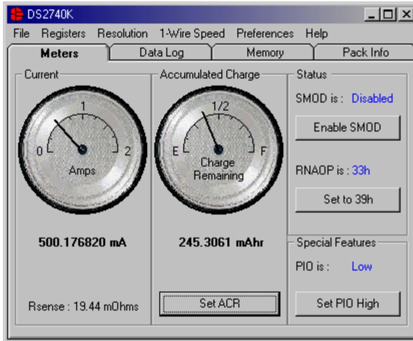
The *Meters Screen* displays the latest real-time measurements of current and accumulated charge with both analog meter readouts and digital values. The sense resistor value used to calculate the current reading is shown in the current section. Left click on it or go to the sense resistor sub-tab under *Pack Info* to change this value.
