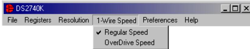
The *1-Wire*<sup>®</sup> *Speed Menu* allows the user to select with which 1-wire speed the device is set. The speed is determined by the state of the pin 1 (OVD pin). If pin 1 has a value of 1, the device communicates with 1-wire overdrive timing. If pin 1 has a value of 0, the device communicates with regular 1-Wire timing.
