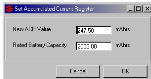
The user can bring up the *Set Accumulated Current Register* window by left clicking the *Set ACR* button. This window allows the user to enter values for the *Accumulated Current Register* and *Rated Battery Capacity* in mA. Clicking the *OK* button will write the *New ACR Value* to the *DS2740's Accumulated Current Register*. The *Rated Battery Capacity* is used to determine full-scale range on the *Accumulated Charge Meter* and is only a software value; it is not stored on the device.
