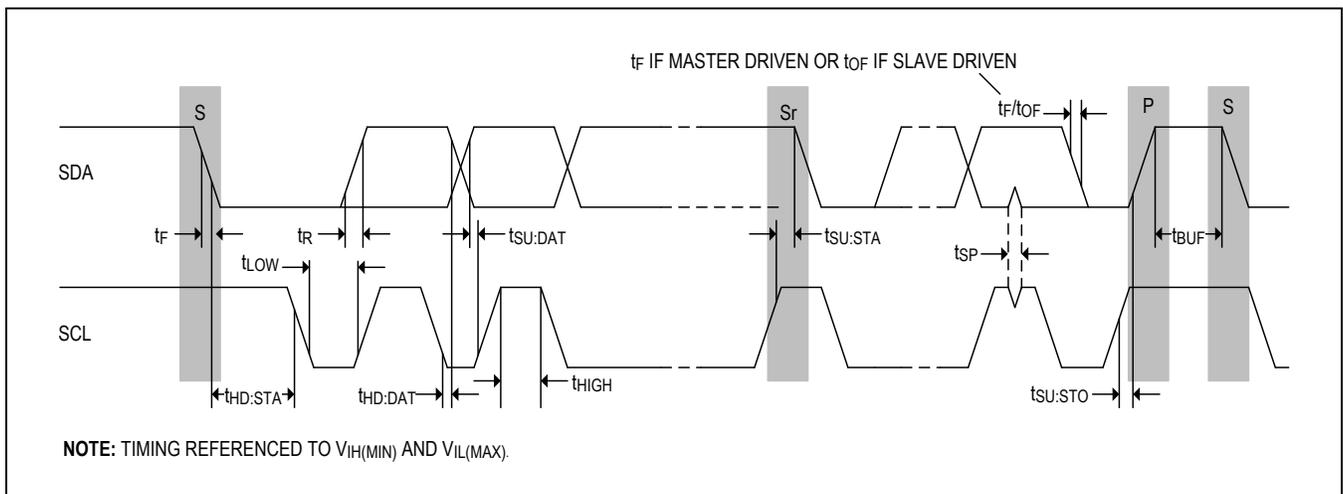
Figure 44: I<sup>2</sup>C Timing Diagram
