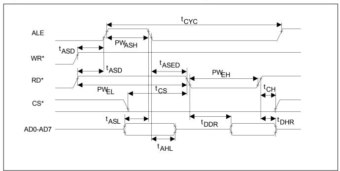
Figure 37-1. Intel Multiplexed Bus Read Timing (BTS = 0/MUX = 1)
