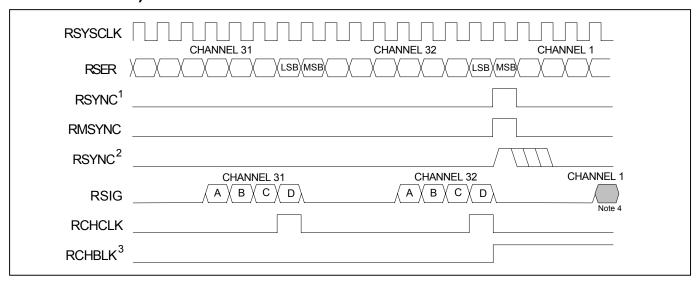
Note 1: RSYNC is in the output mode (IOCR1.4 = 0).
