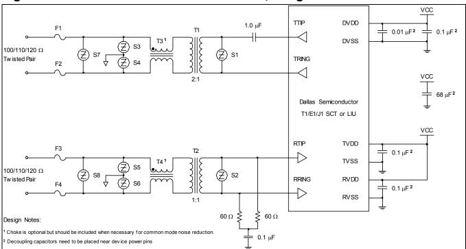
Figure 24-4. Software-Selected Termination, Longitudinal Protection
