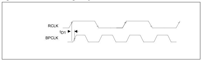
Note 1: If RCLK is 1.544 MHz, BPCLK will be asynchronous.
