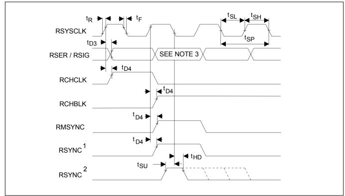
Figure 37-9. Receive-Side Timing, Elastic Store Enabled
