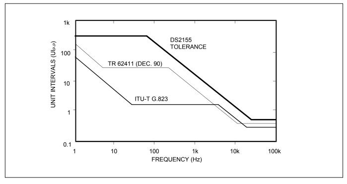
Figure 24-8. Jitter Tolerance (E1 Mode)
