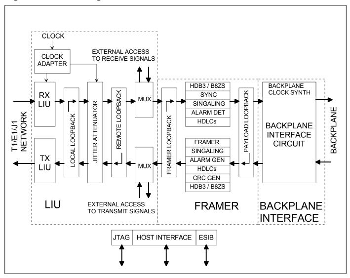
Figure 3-2. Receive and Transmit LIU
