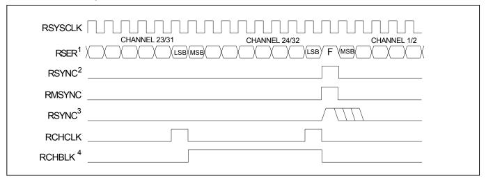
Note 1: Data from the E1 channels 1, 5, 9, 13, 17, 21, 25, and 29 is dropped (channel 2 from the E1 link is mapped to channel 1 of the T1 link, etc.) and the F-bit position is added (forced to on 1).
