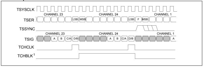
Note 1: TCHBLK is programmed to block channel 24 (if the TPCSI bit is set, then the signaling data at TSIG is ignored during channel 24).
