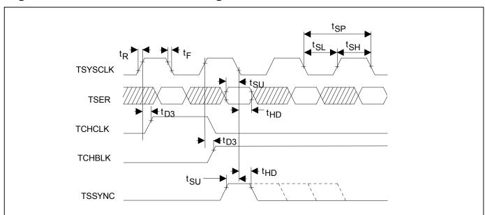
Figure 37-13. Transmit-Side Timing, Elastic Store Enabled
