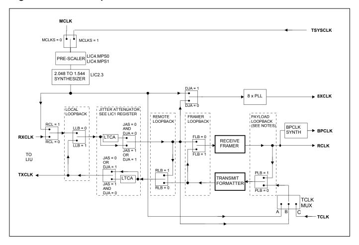
The TCLK MUX is dependent on the state of the TCSS0 and TCSS1 bits in the CCR1 register and the state of the TCLK pin.
