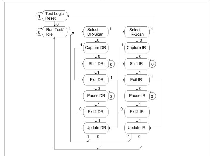
Figure 34-2. TAP Controller State Diagram
