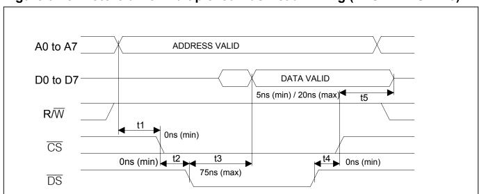
Figure 37-6. Motorola Nonmultiplexed Bus Read Timing (BTS = 1/MUX = 0)
