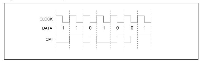
Transmit and receive CMI are enabled through LIC4.7. When this register bit is set, the TTIP pin outputs CMI-coded data at normal levels. This signal can be used to directly drive an optical interface. When CMI is enabled, the user can also use HDB3/B8ZS coding. When this register bit is set, the RTIP pin becomes a unipolar CMI input. The CMI signal is processed to extract and align the clock with data.
