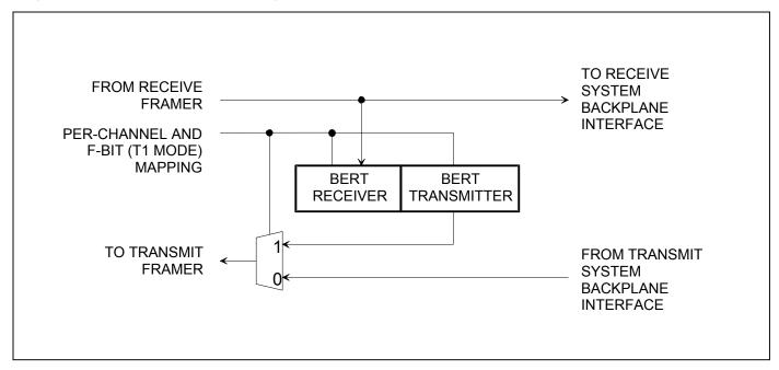
Figure 26-2. Simplified Diagram of BERT in Backplane Direction
