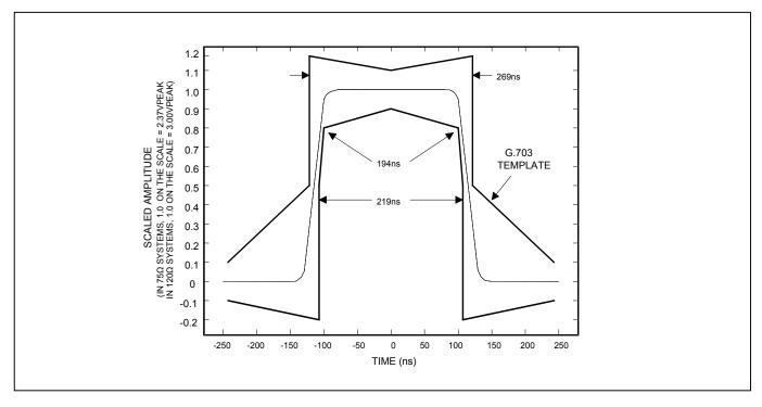
Figure 24-6. T1 Transmit Pulse Template
