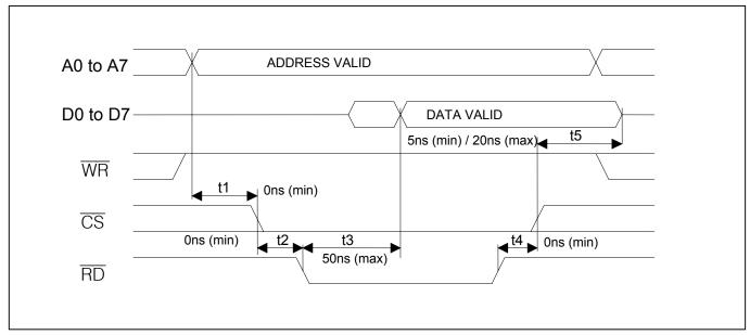
Figure 37-4. Intel Nonmultiplexed Bus Read Timing (BTS = 0/MUX = 0)
