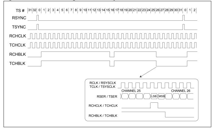
Note 1: RCHBLK or TCHBLK programmed to pulse high during time slots 1 through 15, 17 through 25, and bit 1 of time slot 26.
