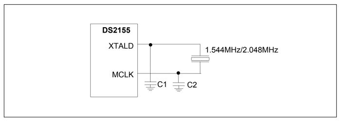
Note 1: C1 and C2 should be 5pF lower than two times the nominal loading capacitance of the crystal to adjust for the input capacitance of the DS2155.
