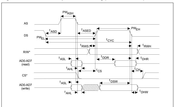
Figure 37-3. Motorola Multiplexed Bus Timing (BTS = 1/MUX = 1)
