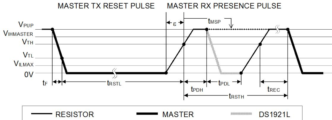
After the bus master has released the line it goes into receive mode (RX). Now, the 1-Wire bus is pulled to  $V_{PUP}$  via the pull-up resistor or, in case of a DS2480B driver, by active circuitry. When the threshold  $V_{TH}$  is crossed, the DS1921L waits for  $t_{PDH}$  and then transmits a Presence Pulse by pulling the line low for  $t_{PDL}$ . To detect a presence pulse, the master must test the logical state of the 1-Wire line at  $t_{MSP}$ .
