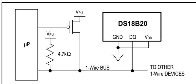
Figure 6. Supplying the Parasite-Powered DS18B20 During Temperature Conversions
