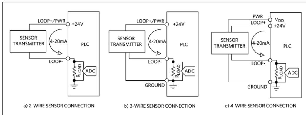
Figure 1. Sensor transmitter connection types.
