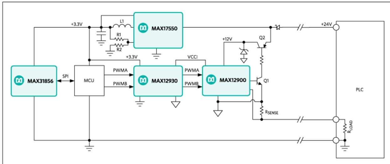
Figure 4. A 3-wire sensor transmitter with DC-DC converter.
