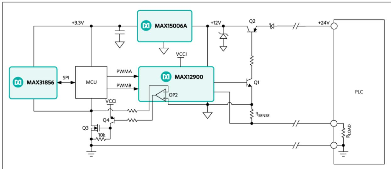
Figure 5. A 3-wire sensor transmitter with linear regulator.
