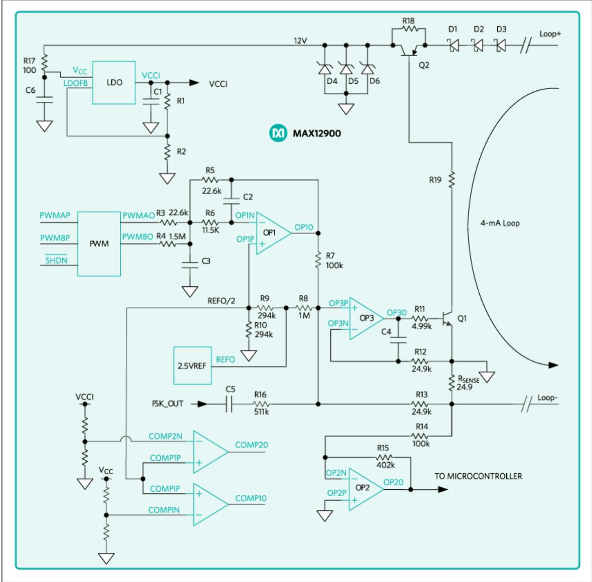
Figure 3. Configuration of loop-powered 4-20mA transmitter using MAX12900.
