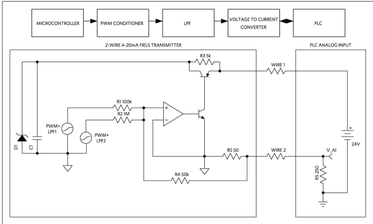
Figure 2. Block diagram and model of loop-powered sensor using MAX12900.
