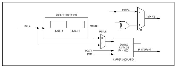
Figure 2. IR Transmit Carrier Generation and Carrier Modulator Control
