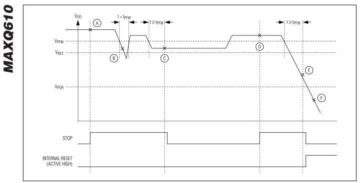
Figure 12. Stop Mode Power-Fail Detection States with Power-Fail Monitor Enabled
