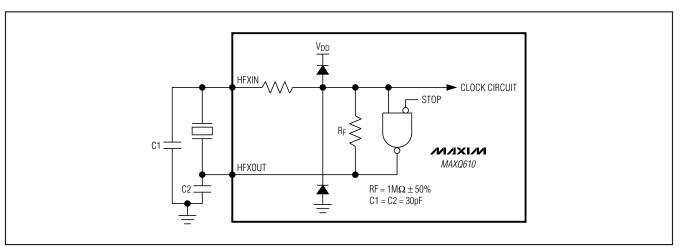
Figure 9. On-Chip Oscillator
