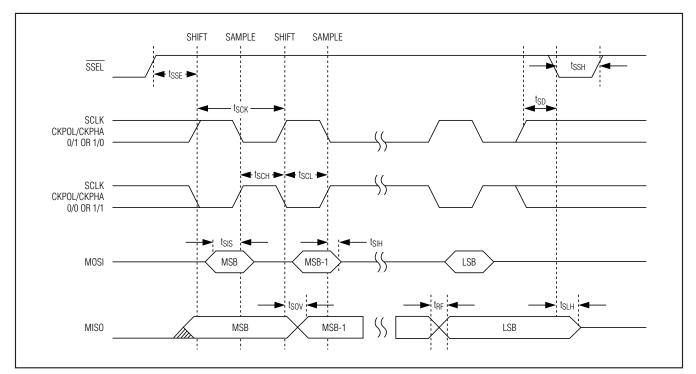
Figure 8. SPI Slave Communication Timing
