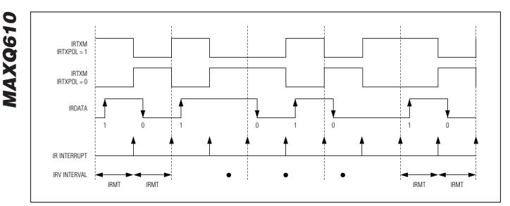
Figure 4. External IRTXM (Modulator) Output
