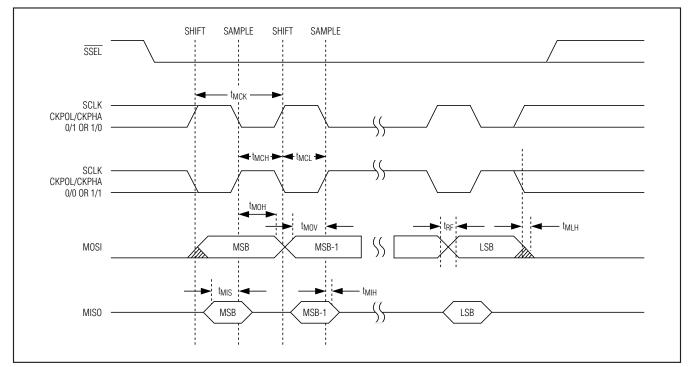
Figure 7. SPI Master Communication Timing
