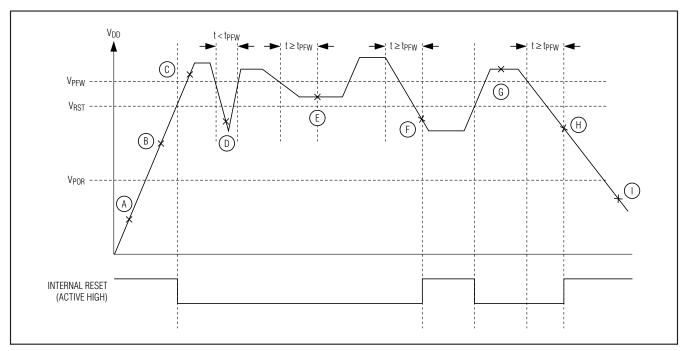
Figure 11. Power-Fail Detection During Normal Operation
