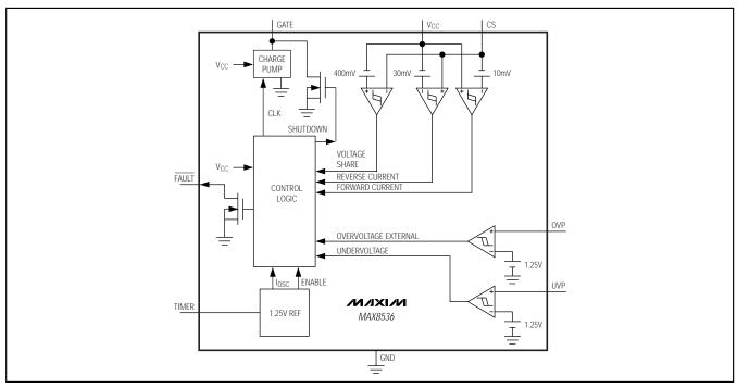
Figure 2. MAX8536 Functional Diagram
