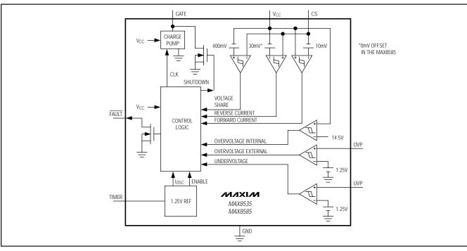
Figure 1. MAX8535/MAX8585 Functional Diagram
