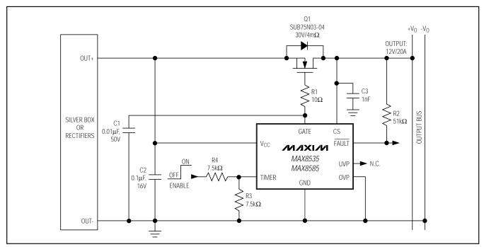
Figure 5. Typical Application Circuit for 12V/20A Output without OVP and UVP
