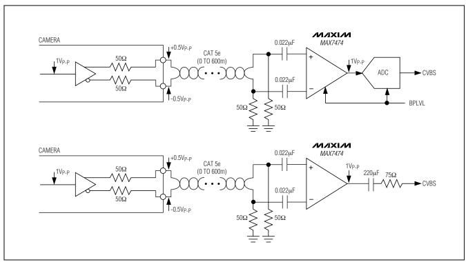
Figure 1. Typical Input and Output Connections
