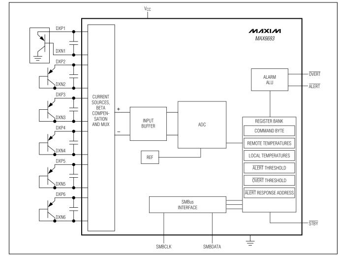
Figure 1. Internal Block Diagram
