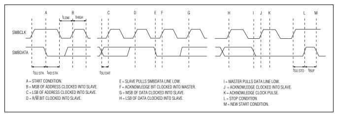
Figure 4. SMBus Read-Timing Diagram
