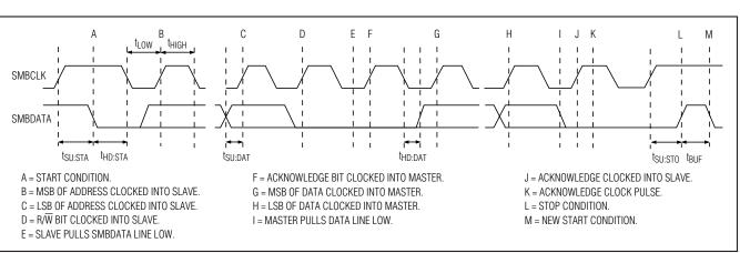
Figure 3. SMBus Write-Timing Diagram
