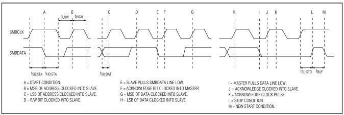
Figure 3. SMBus Write-Timing Diagram
