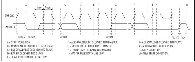
Figure 4. SMBus Read-Timing Diagram
