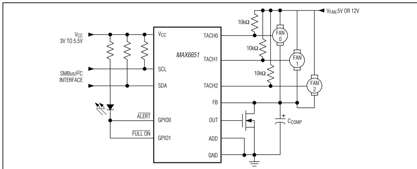
Figure 7. Using the MAX6651 to Control Parallel Fans
