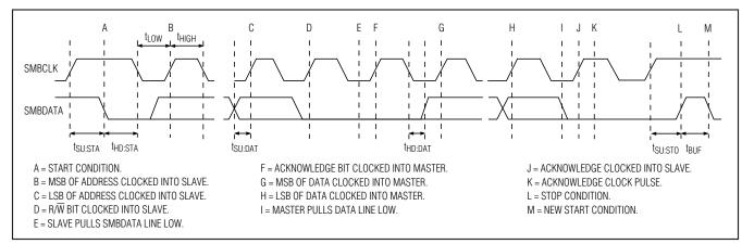
Figure 4. SMBus Read-Timing Diagram
