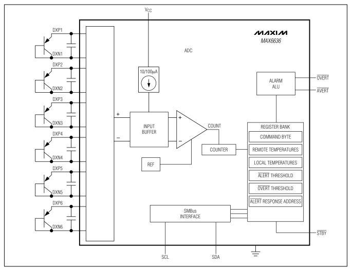
Figure 1. Internal Block Diagram
