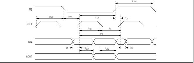
Figure 5. Detailed Serial-Interface Timing Diagram
