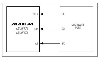
Figure 3. Connections for MICROWIRE
