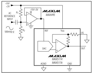
Figure 11. AC Reference Input Circuit
