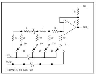
Figure 1. Simplified DAC Circuit Diagram
