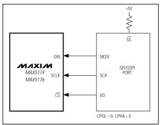
Figure 2. Connections for SPI and QSPI Standards
