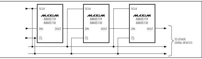
Figure 9. Daisy-Chaining MAX5174/MAX5175 Devices
