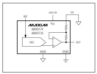
Figure 6. Unipolar Output Circuit (Rail-to-Rail)
