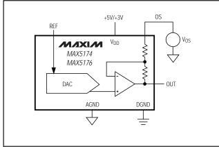
Figure 7. Setting OS for Output Offset
