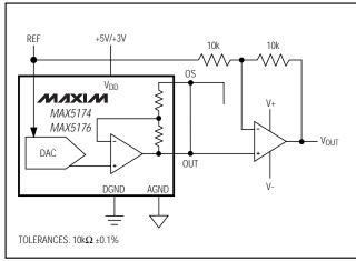
Figure 8. Bipolar Output Circuit
