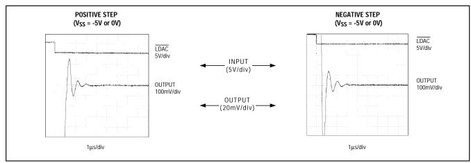
Figure 2. Positive and Negative Settling Times
