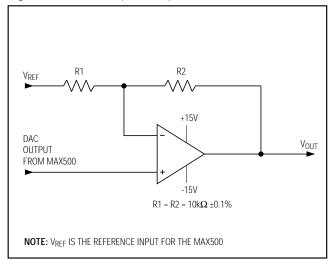
Figure 9. Bipolar Output Circuit
