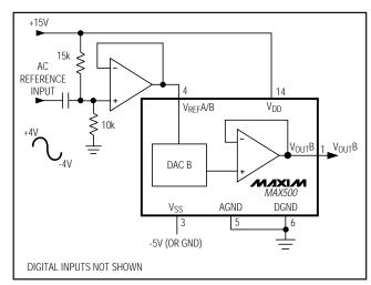
Figure 11. AC Reference Input Circuit
