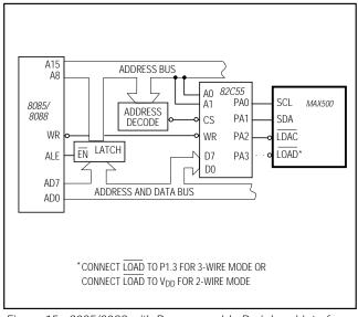
Figure 15. 8085/8088 with Programmable Peripheral Interface
