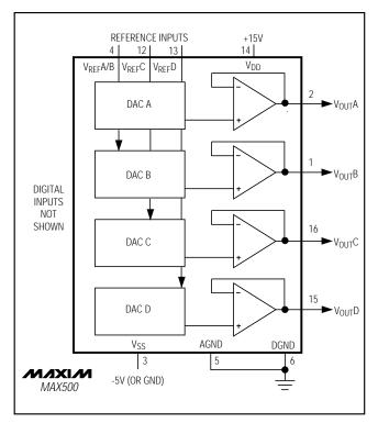
Figure 8. MAX500 Unipolar Output Circuit
