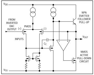
Figure 4. Simplified Output Buffer Circuit
