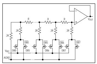
Figure 1. Simplified DAC Circuit Diagram
