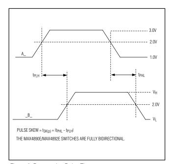
Figure 3. Propagation Delay Times
