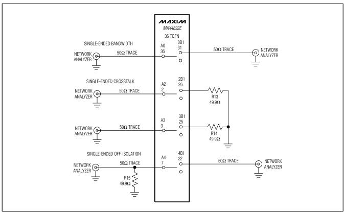
Figure 1. Single-Ended Bandwidth, Crosstalk, and Off-Isolation
