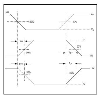
Figure 2. Turn-On and Turn-Off Times
