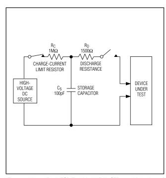
Figure 5. Human Body ESD Test Model (MIL-STD-883, Method 3015)
