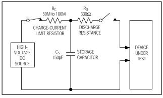
Figure 10. IEC 1000-4-2 ESD Test Model
