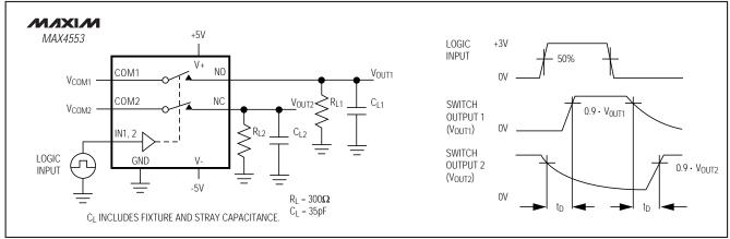
Figure 2. Break-Before-Make Interval (MAX4553 only)
