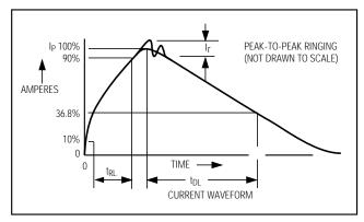
Figure 9. Human Body Model Current Waveform
