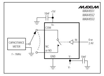
Figure 6. Channel Off-Capacitance
