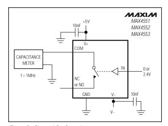
Figure 7. Channel On-Capacitance
