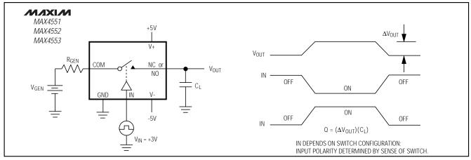
Figure 3. Charge Injection
