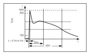
Figure 11. IEC 1000-4-2 ESD Generator Current Waveform
