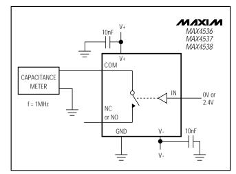
Figure 7. Channel-On Capacitance
