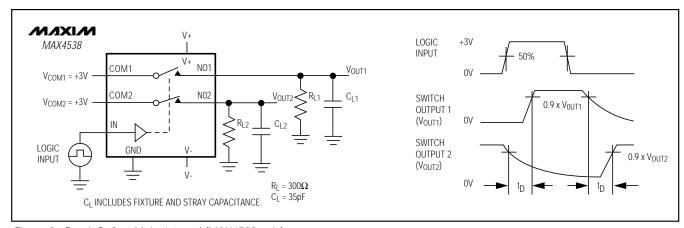
Figure 2. Break-Before-Make Interval (MAX4538 only)
