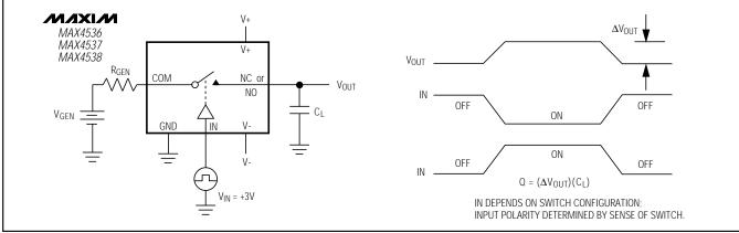
Figure 3. Charge Injection
