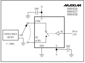
Figure 6. Channel-Off Capacitance
