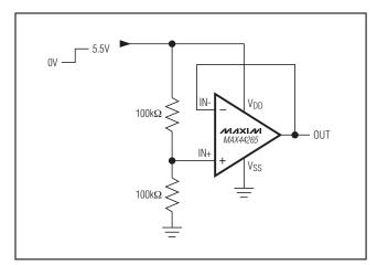
Figure 3. Power-Up Test Configuration
