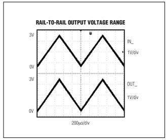
Figure 1. Rail-to-Rail Output Voltage Range
