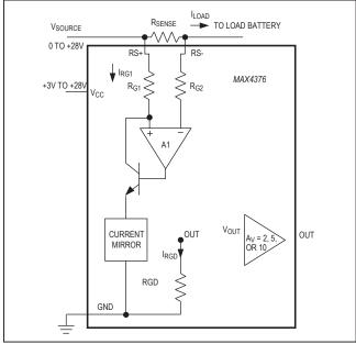
Figure 1. Functional Diagram
