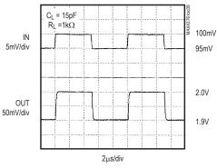
MAX4376H SMALL-SIGNAL TRANSIENT RESPONSE (V<sub>SENSE</sub> = 95mV to 100mV)
