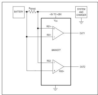
Figure 2. Bidirectional Current Monitor
