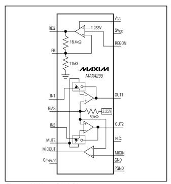
Figure 2. MAX4299 Block Diagram
