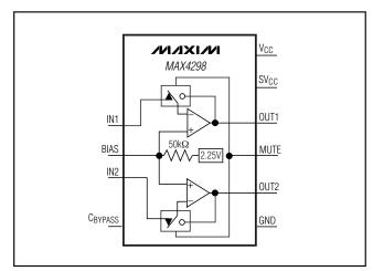
Figure 1. MAX4298 Block Diagram
