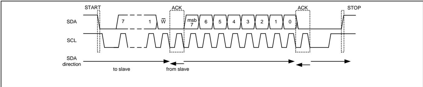
Figure 26. Write Transaction
