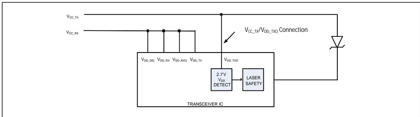
Figure 13.  $V_{DD\_TXO}$  Configured to Assert Laser Shutdown
