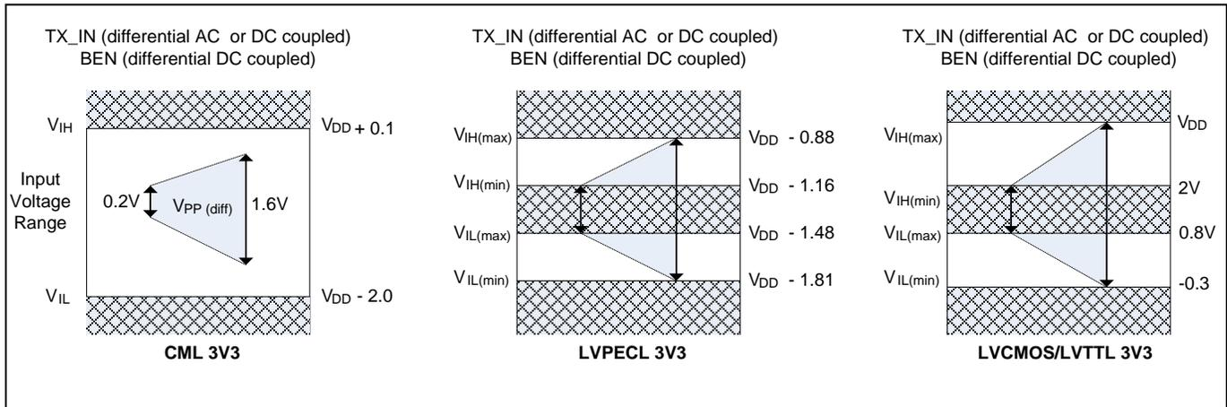
Typical I/O ranges for TX\_IN and BEN are shown. TX\_IN and BEN inputs are also compatible with HSTL and SSTL for low voltage operation.
