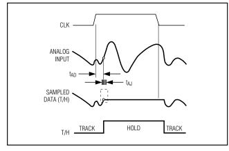
Figure 16. T/H Aperture Timing
