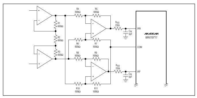
Figure 13. Rx ADC DC-Coupled Differential Drive
