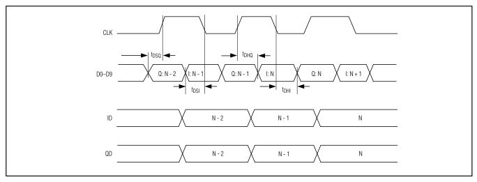
Figure 6. Tx DAC System Timing Diagram
