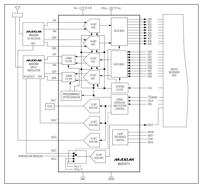
Figure 14. Typical Application Circuit for CDMA Radio
