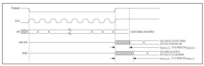
Figure 8. Mode-Recovery Timing Diagram
