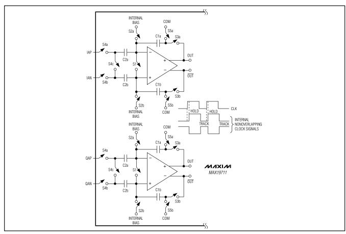
Figure 1. Rx ADC Internal T/H Circuits
