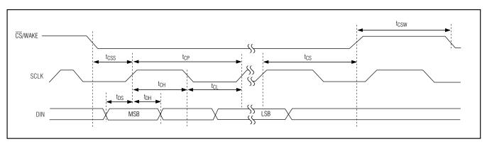
Figure 7. Serial-Interface Timing Diagram
