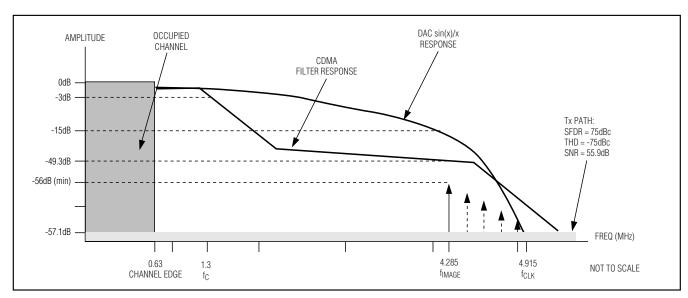
Figure 4. TD-SCDMA Filter Frequency Response
