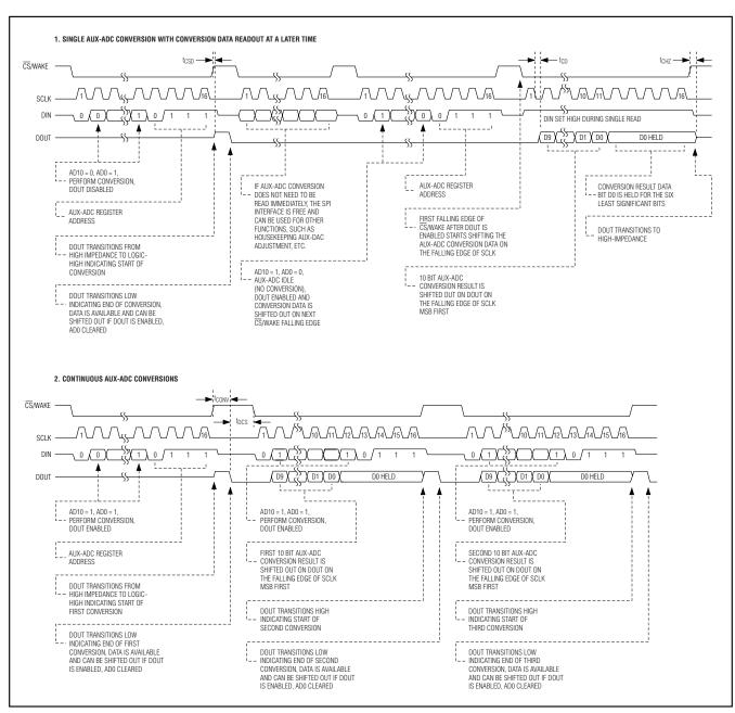
Figure 9. Aux-ADC Conversions Timing
