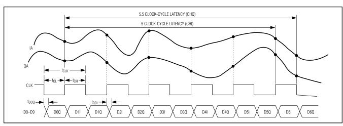
Figure 3. Rx ADC System Timing Diagram
