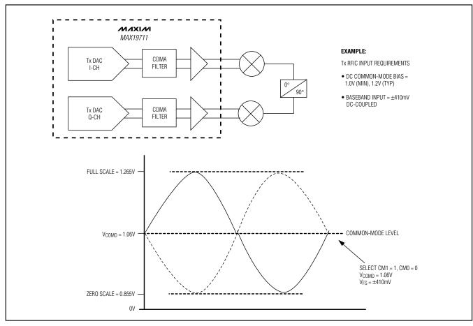
Figure 5. Tx DAC Common-Mode DC Level at IDN, IDP or QDN, QDP Differential Outputs
