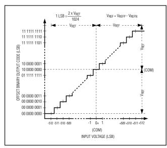
Figure 2. Rx ADC Transfer Function
