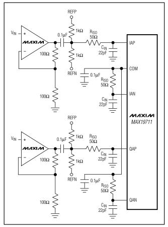
Figure 12. Single-Ended Drive for Rx ADC
