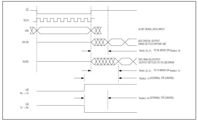
Figure 7. Mode-Recovery Timing Diagram
