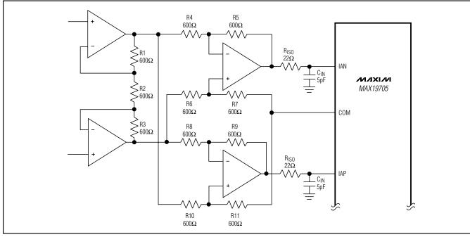
Figure 11. Rx ADC DC-Coupled Differential Drive
