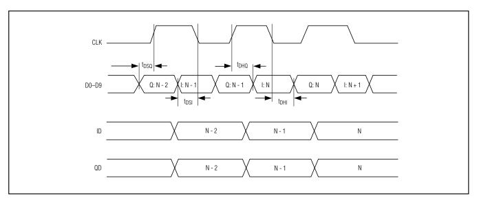
Figure 5. Tx DAC System Timing Diagram
