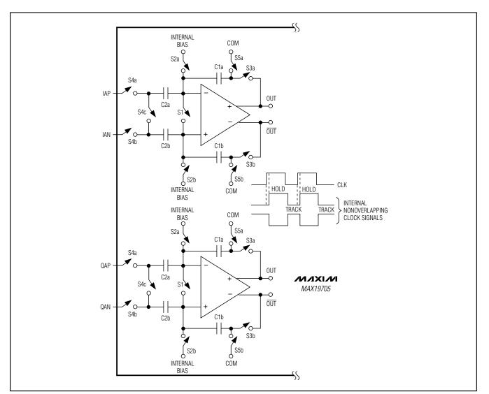
Figure 1. Rx ADC Internal T/H Circuits
