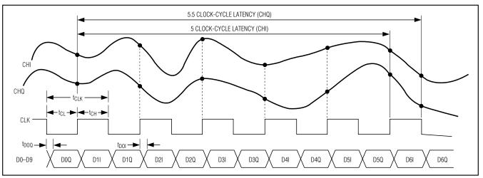
Figure 3. Rx ADC System Timing Diagram
