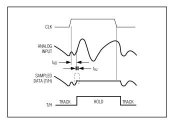
Figure 14. T/H Aperture Timing
