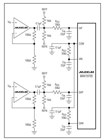
Figure 10. Single-Ended Drive for Rx ADC
