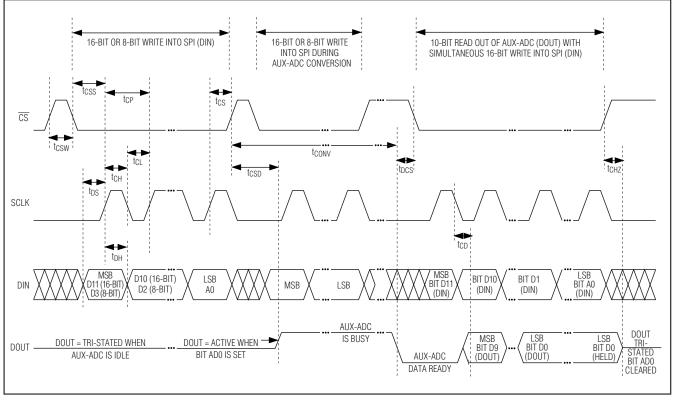
Figure 6. Serial-Interface Timing Diagram
