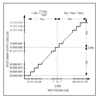
Figure 2. Rx ADC Transfer Function
