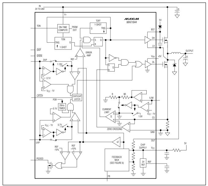
Figure 2. MAX1844 Functional Diagram
