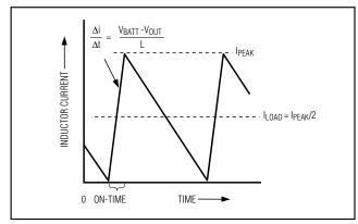
Figure 3. Pulse-Skipping/Discontinuous Crossover Point
