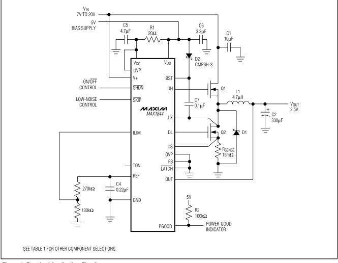
Figure 1. Standard Application Circuit
