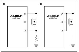
Figure 8. Current-Sense Circuits
