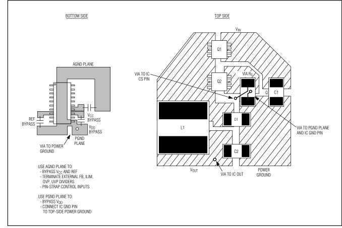
Figure 9. Power-Stage PC Board Layout Example
