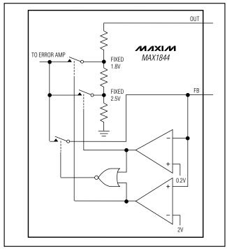
Figure 6. Feedback Mux
