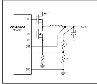
Figure 7. Setting VOUT with a Resistor-Divider
