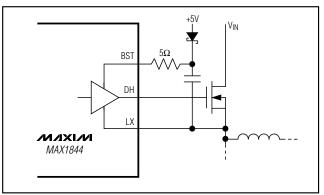
Figure 5. Reducing the Switching-Node Rise Time
