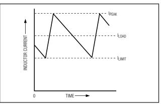
Figure 4. "Valley" Current-Limit Threshold Point
