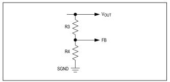
Figure 2. Setting the Output Voltage
