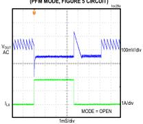
MAX17504 3.3V OUTPUT LOAD CURRENT STEPPED FROM 5mA TO 1.75A (PFM MODE, FIGURE 4 CIRCUIT)
