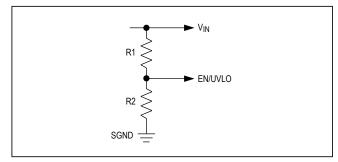
Figure 1. Setting the Input Undervoltage Lockout
