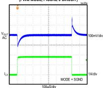
MAX17504 5V OUTPUT LOAD CURRENT STEPPED FROM 5mA TO 1.75A (PFM MODE, FIGURE 3 CIRCUIT)
