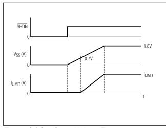
Figure 5. Soft-Start Current Limit over Time
