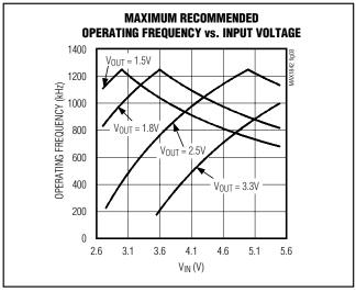
Figure 3. Maximum Recommended Operating Frequency vs. Input Voltage
