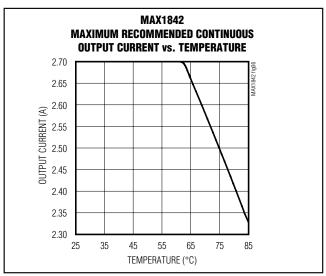
Figure 6. MAX1842 Maximum Recommended Continuous Output Current vs. Temperature
