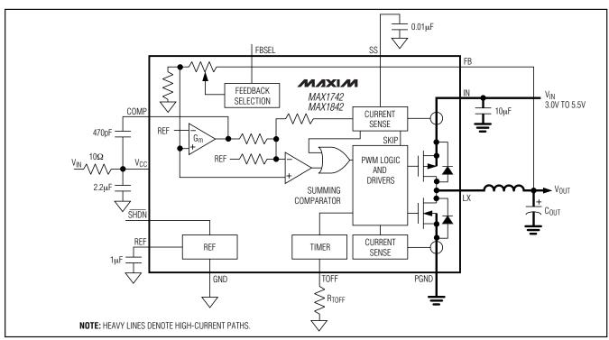
Figure 2. Functional Diagram
