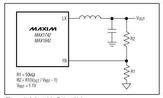
Figure 4. Adjustable Output Voltage
