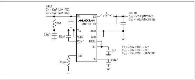
Figure 1. Typical Circuit
