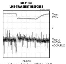
$I_{OUT}=2.5\text{A},\ V_{OUT}=1.5\text{V},\ R_{TOFF}=100\text{k}\Omega,\ L=2.2\mu\text{H}$
