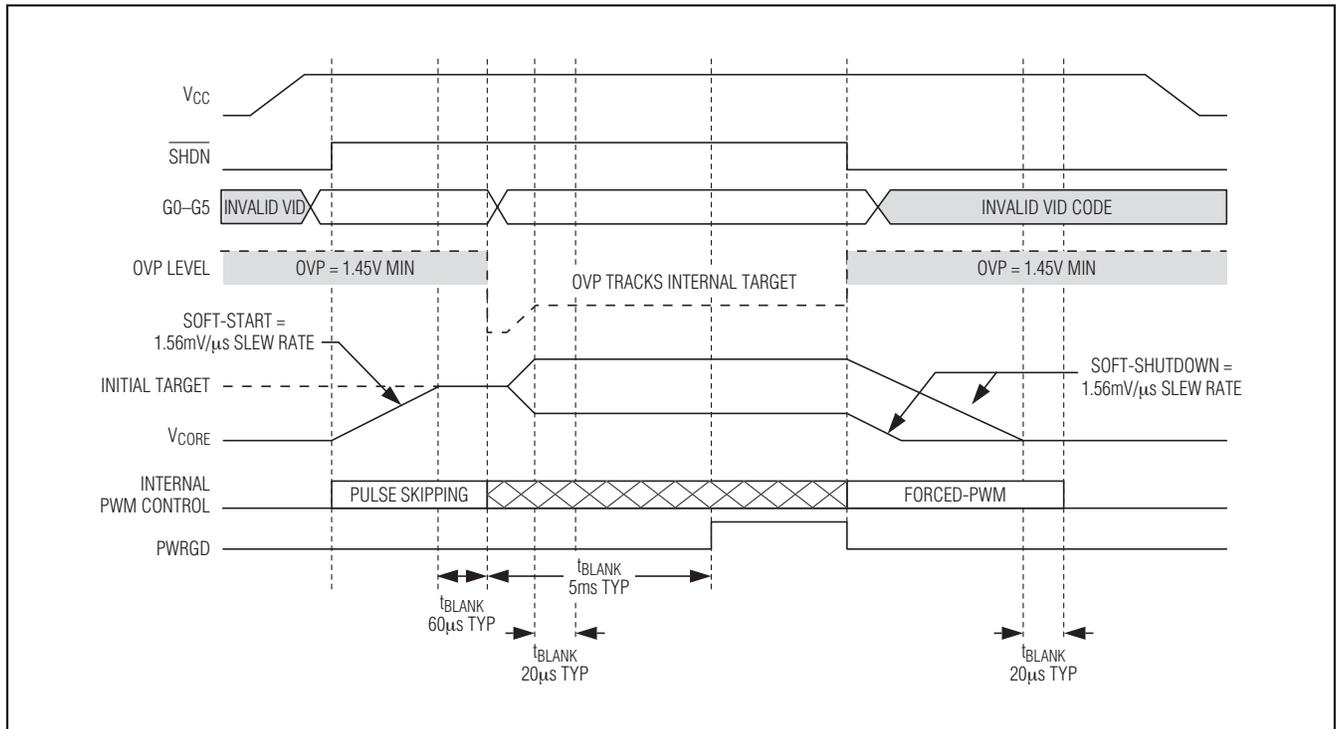
Figure 6. Power-Up and Shutdown Sequence Timing Diagram
