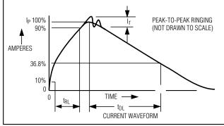
Figure 3b. Human Body Model Current Waveform
