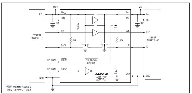
Figure 2. Typical Application Circuit and Functional Diagram
