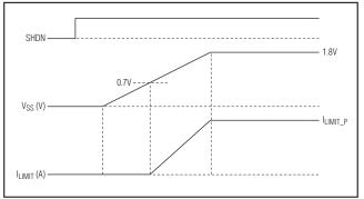
Figure 3. Soft-Start Current Limit
