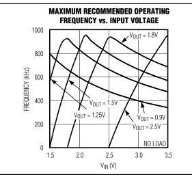
Figure 6. Maximum Operating Frequency vs. Input Voltage
