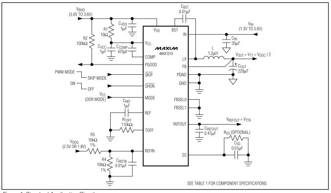
Figure 1. Standard Application Circuit
