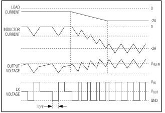
Figure 4. Sink-Mode Waveforms
