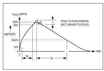
Figure 3. Human Body Current Waveform
