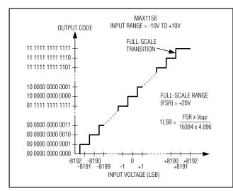
Figure 9. MAX1158 Transfer Function
