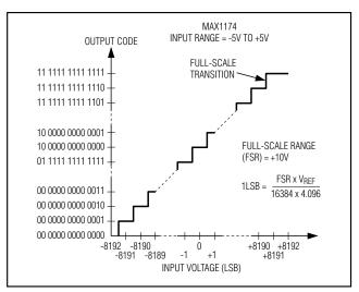
Figure 10. MAX1174 Transfer Function
