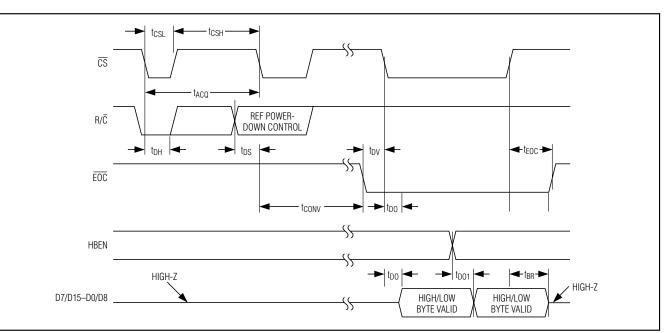
Figure 2. MAX1156/MAX1158/MAX1174 Timing Diagram
