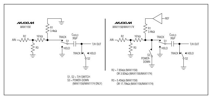
Figure 4. Equivalent Input Circuit
