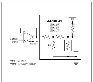
Figure 11. MAX1156/MAX1158/MAX1174 Fast-Settling Input Buffer
