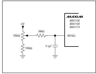
Figure 7. MAX1156/MAX1158/MAX1174 Reference Adjust Circuit
