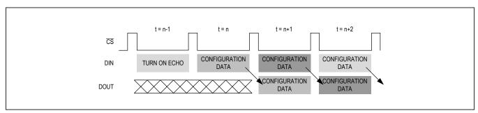
Figure 8. Echo Back the Configuration Data
