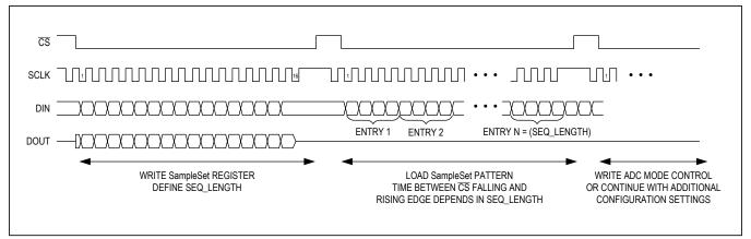
Figure 10. SampleSet Timing Diagram
