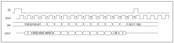
Figure 2c. External Clock Mode Timing Diagram with CHAN\_ID=0
