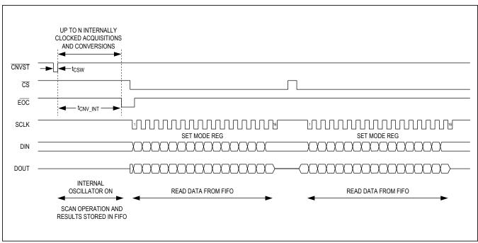
Figure 6. Internal Conversions with CNVST
