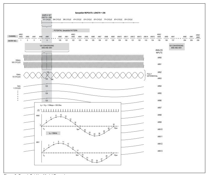
Figure 9. SampleSet Use-Model Example
