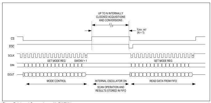
Figure 7. Internal Conversions with SWCNV
