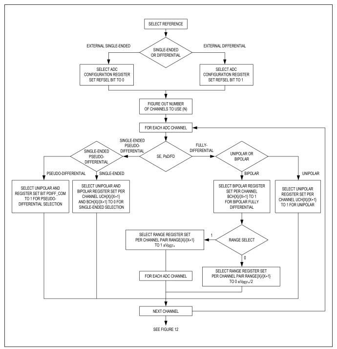
Figure 11. ADC Programming Sequence
