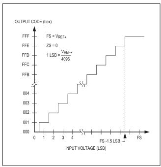
Figure 4. Unipolar Transfer Function for 12-Bit Resolution
