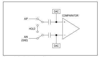
Figure 3. Equivalent Input Circuit
