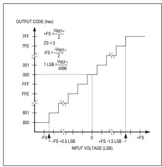
Figure 5. Bipolar Transfer Function for 12-Bit Resolution
