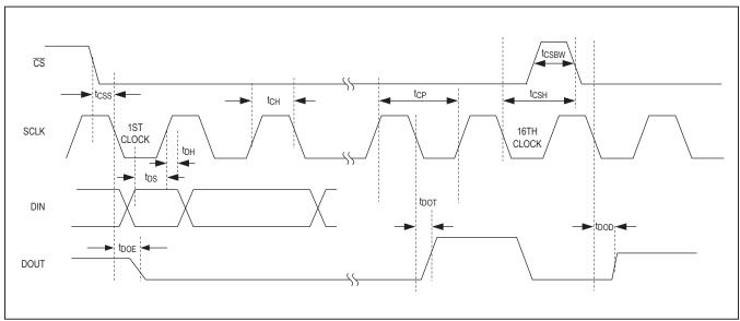
Figure 1. Detailed Serial-Interface Timing Diagram
