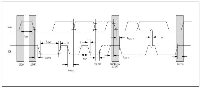
Figure 6. 2-Wire AC Characteristics
