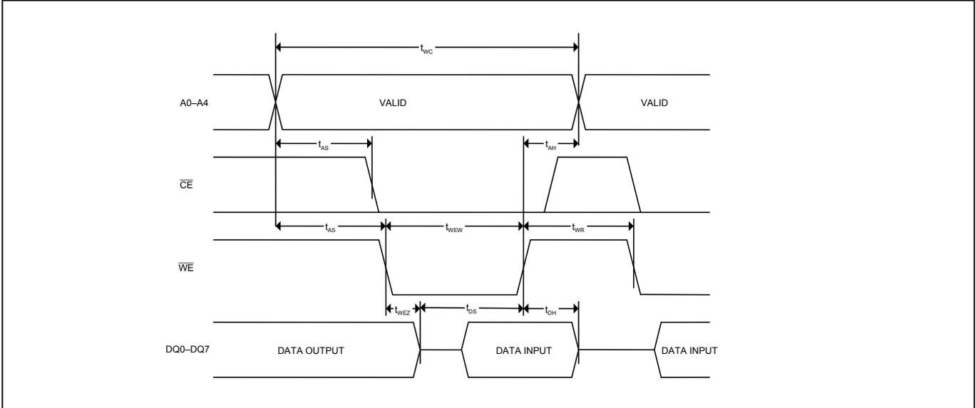
**Figure 3. Write Cycle Timing, Chip-Enable Controlled**
