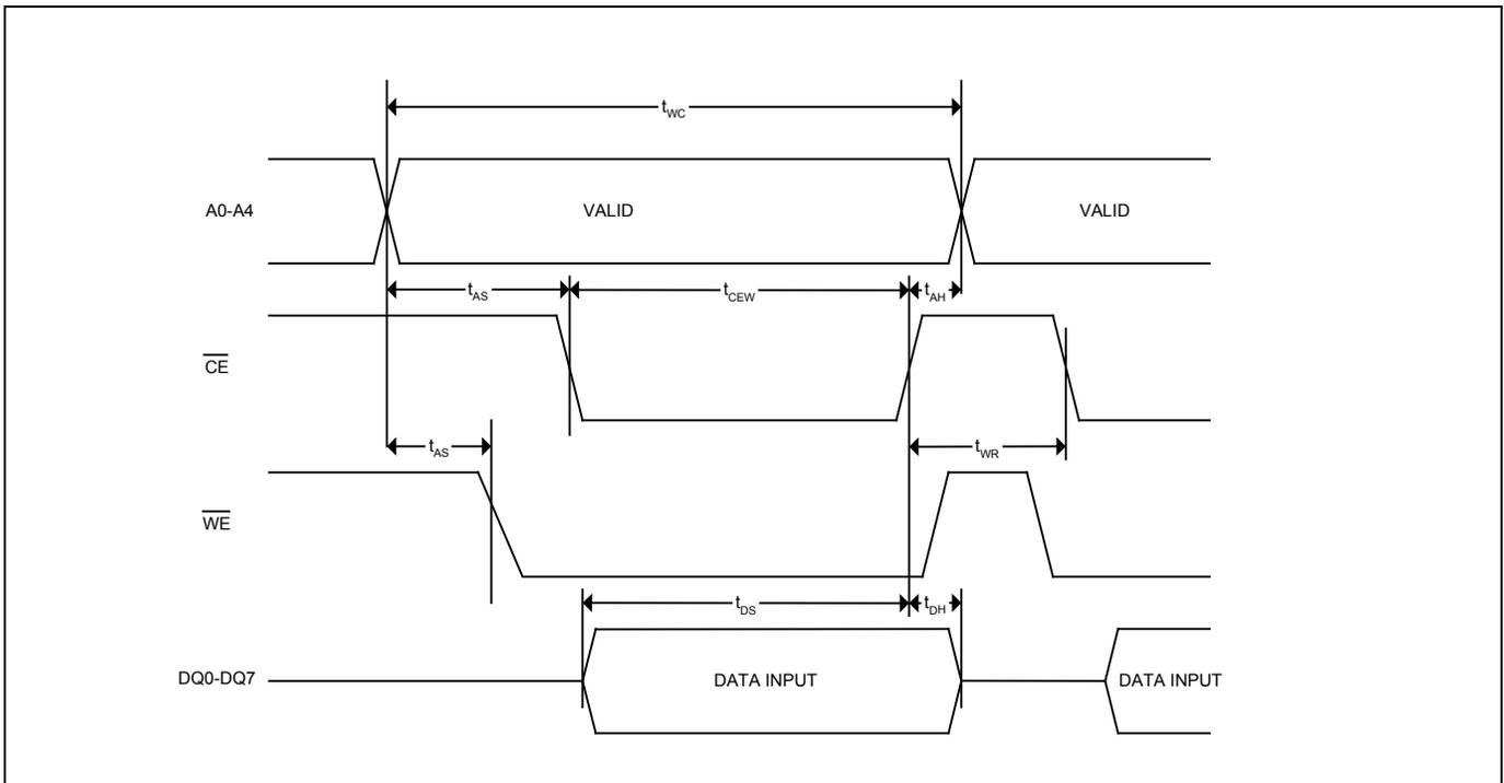
Figure 4. Burst Mode Timing Waveform
