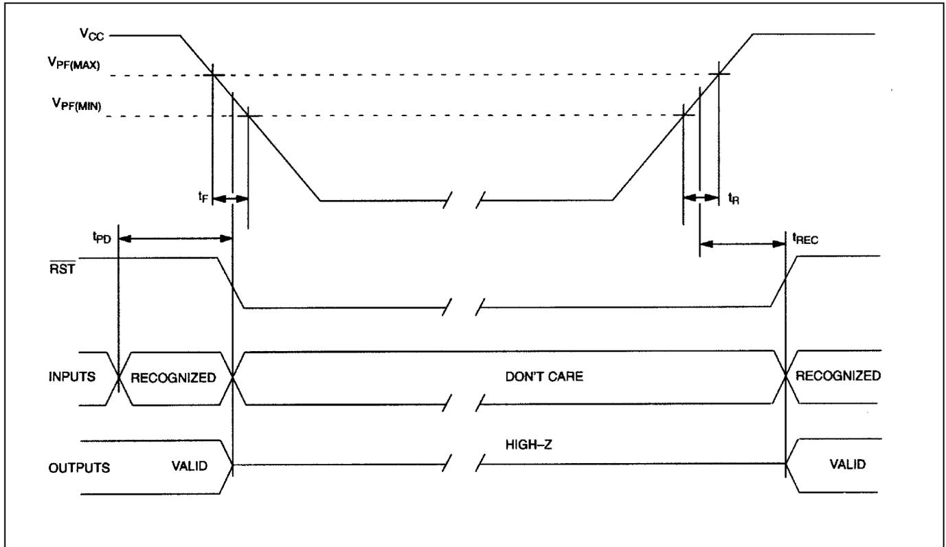
Figure 6. 5V Power-Up/Down Waveform Timing
