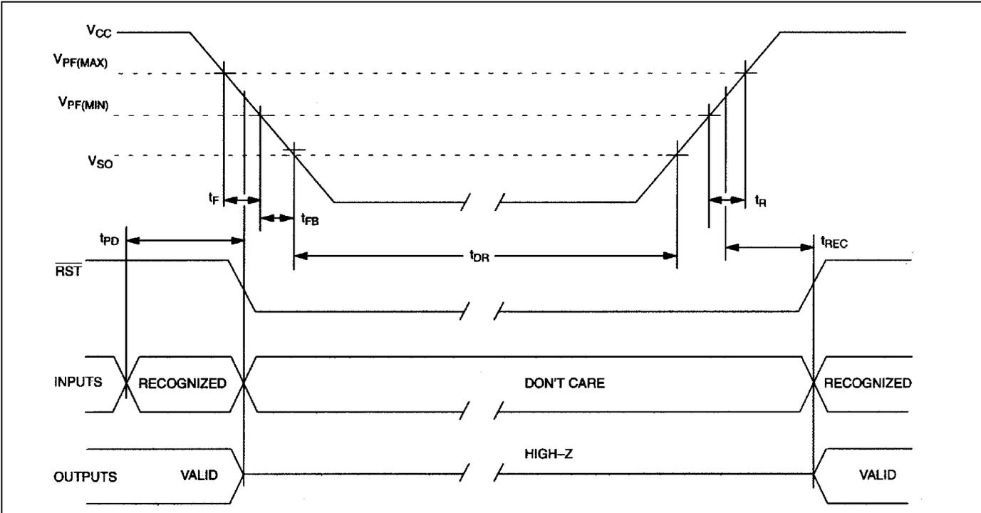
**Warning:** Under no circumstances are negative undershoots, of any amplitude, allowed when device is in battery-backup mode.
