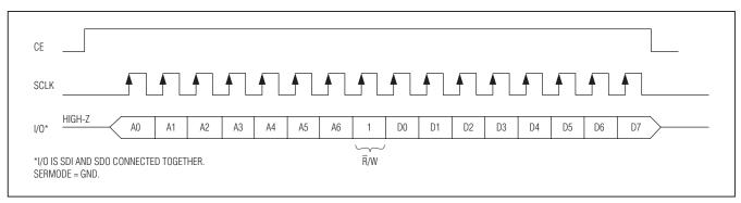
Figure 7. 3-Wire Single-Byte Write
