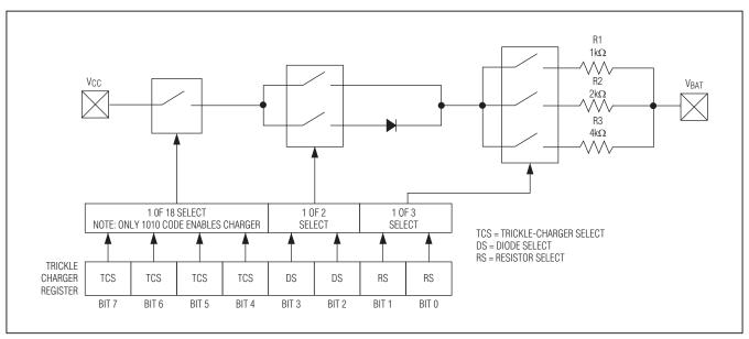
Figure 2. Trickle Charger Block Diagram
