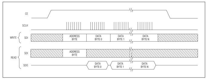
Figure 6. SPI Multibyte Burst Transfer
