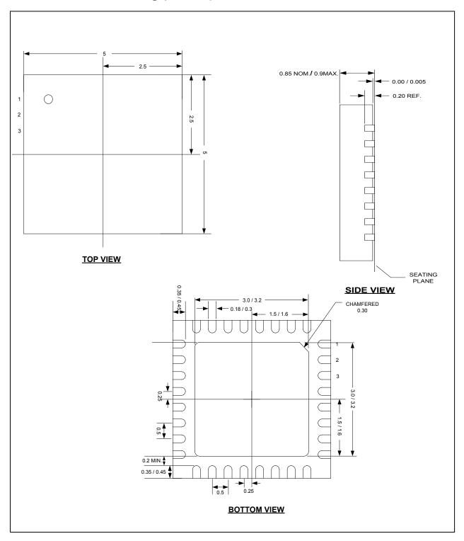
Figure 11: 32QFN Mechanical Drawing
