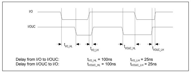
Figure 7: I/O – I/OUC Delays Timing Diagram
