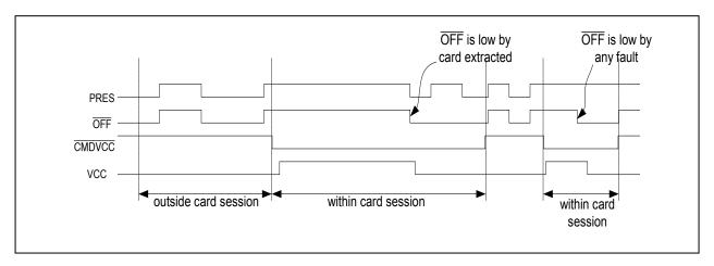
Figure 5: Timing Diagram - Management of the Interrupt Line OFF
