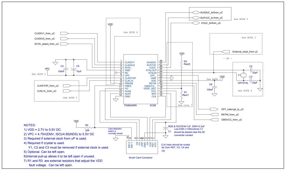
Figure 8: 73S8024RN - Typical Application Schematic
