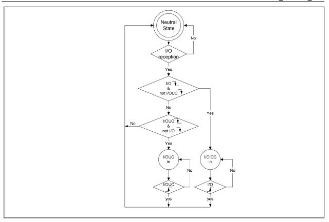
Figure 6: I/O and I/OUC State Diagram
