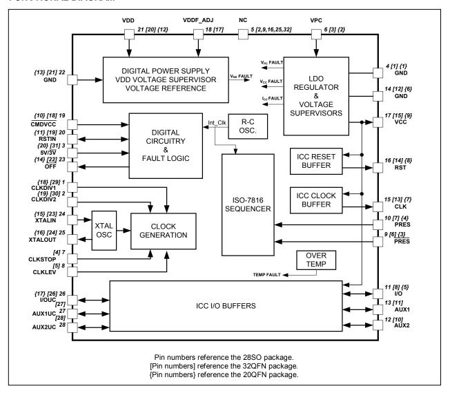
Figure 1: 73S8024RN Block Diagram
