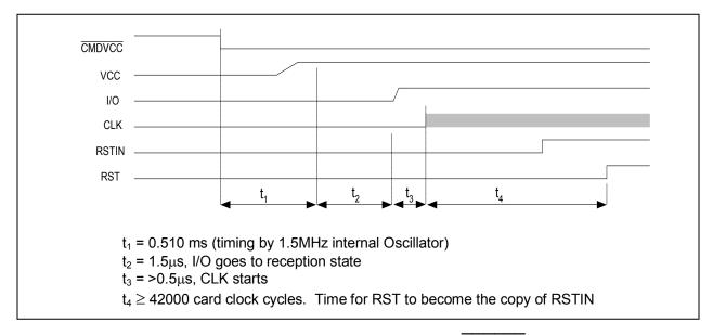
Figure 2: Activation Sequence – RSTIN Low When CMDVCC Goes Low
