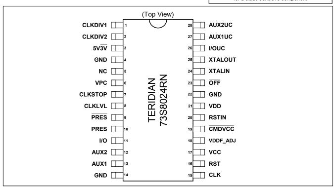
Figure 14: 28SO 73S8024RN Pin Out
