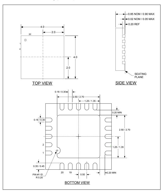
Figure 9: 20QFN Mechanical Drawing
