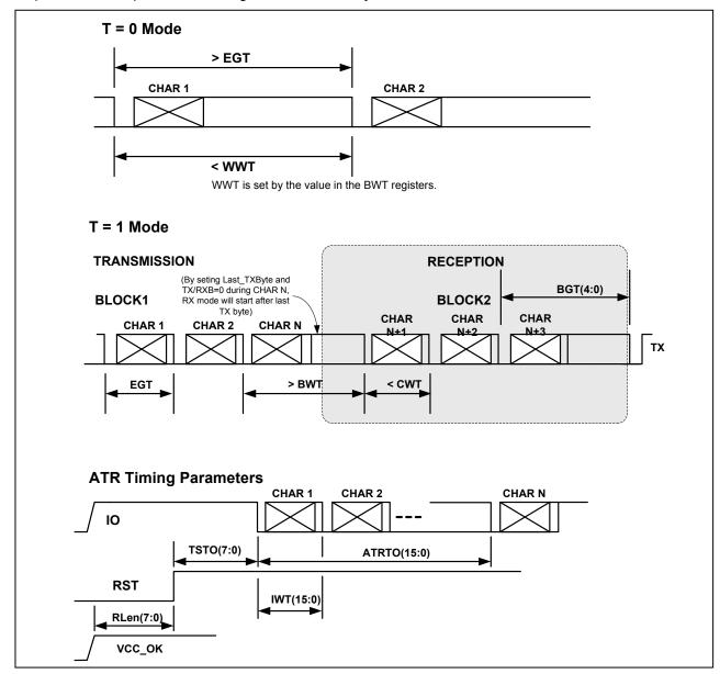
Figure 18: Guard, Block, Wait and ATR Time Definitions
