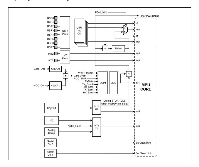
**Figure 8: External Interrupt Configuration**
