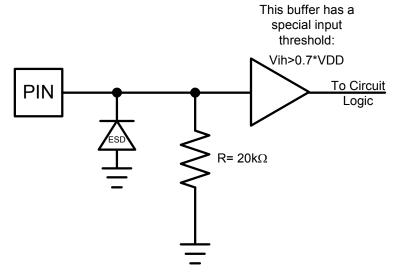
Figure 35: Test and Security Pin Circuit
