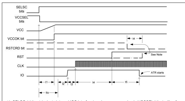
t1: SELSC.1 bit set (selects internal ICC interface) and a non-zero value in VCCSEL bits (calling for a value of Vcc of 1.8, 3.0, or 5.0 volts) will begin the activation sequence. t1 is the time for Vcc to rise to acceptable level, declared as Vcc OK (bit VCCOK gets set). This time depends on filter capacitor value and card lcc load.
