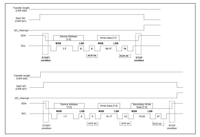
Figure 9: I<sup>2</sup>C Write Mode Operation
