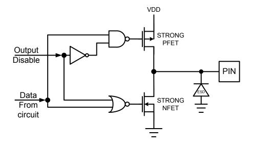
Figure 28: Digital Output Circuit
