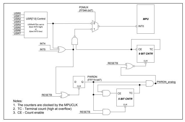
Figure 6: Detail of Power-Down Interrupt Logic
