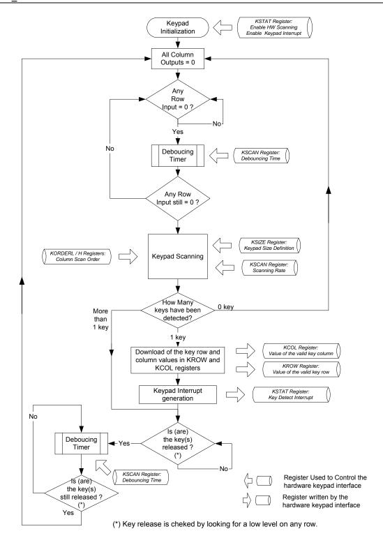
Figure 12: Keypad Interface Flow Chart
