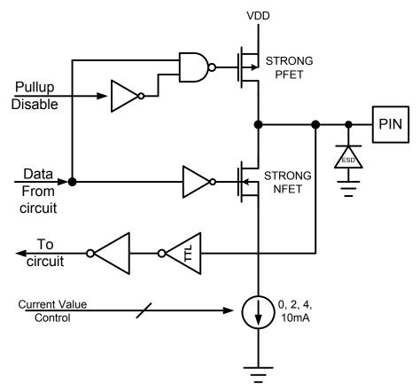
Figure 34: LED Circuit
