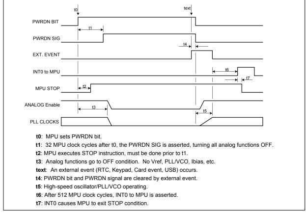
Figure 7: Power-Down Sequencing
