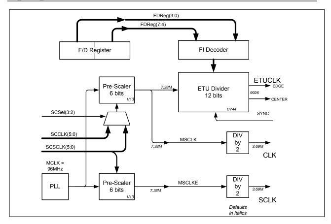
Figure 17: Smart Card CLK and ETU Generation
