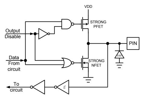
Figure 27: Digital I/O Circuit
