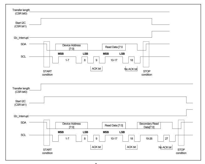
Figure 10: I<sup>2</sup>C Read Operation
