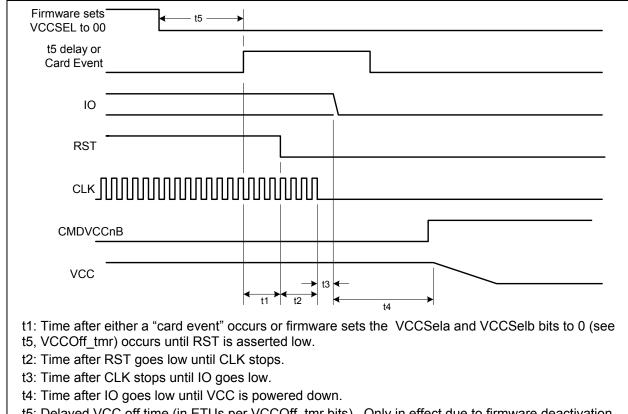
Figure 15: Asynchronous Activation Sequence Timing
