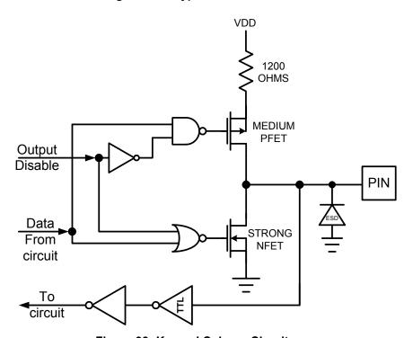
Figure 33: Keypad Column Circuit
