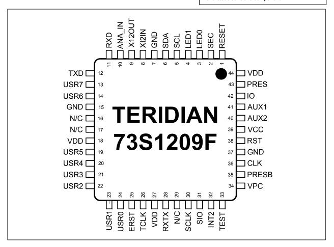
Figure 42: 73S1209F Pinout
