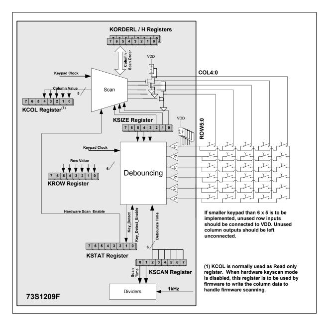
Figure 11: Simplified Keypad Block Diagram
