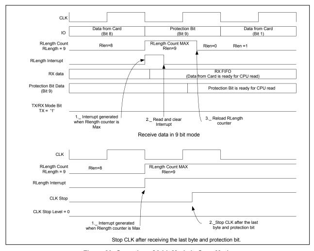
Figure 23: Operation of 9-bit Mode in Sync Mode
