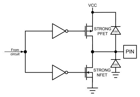
Figure 37: Smart Card Output Circuit
