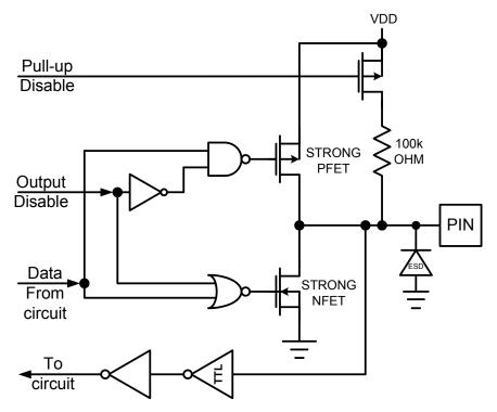
Figure 32: Keypad Row Circuit
