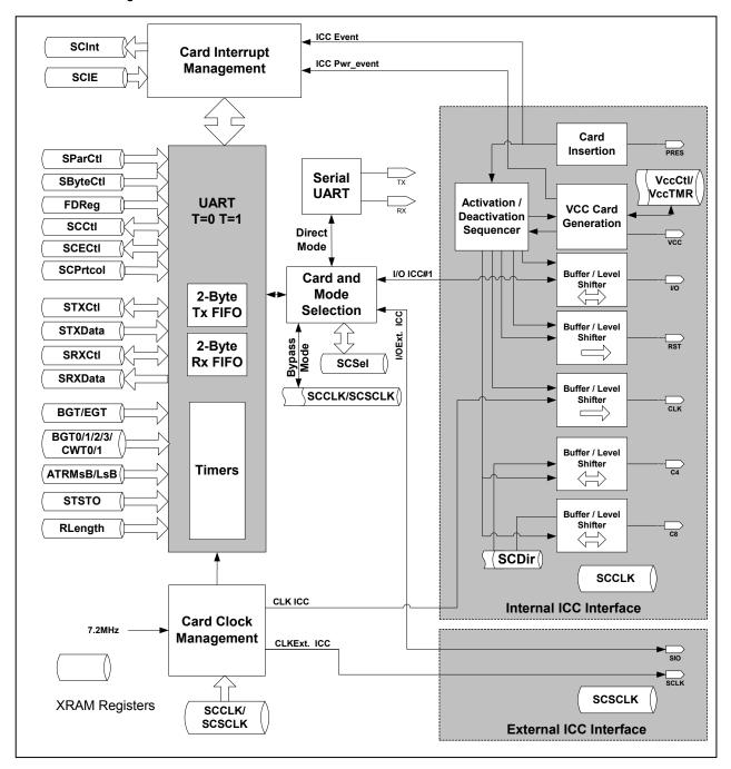
Figure 13: Smart Card Interface Block Diagram
