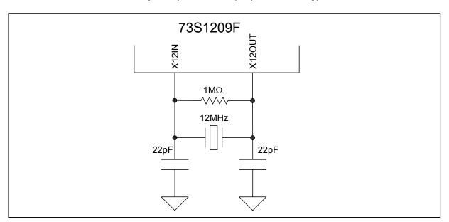
Note: The crystal should be placed as close as possible to the IC, and vias should be avoided.
