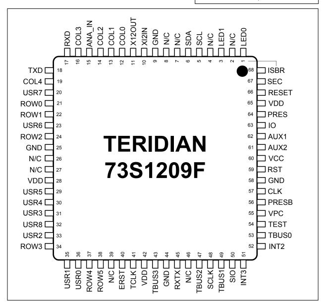
Figure 41: 73S1209F Pinout
