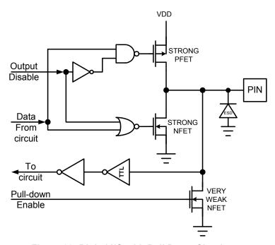
Figure 30: Digital I/O with Pull Down Circuit
