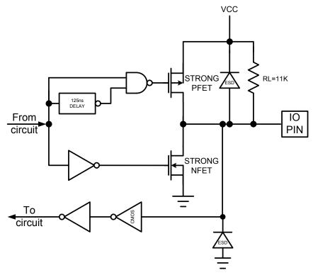
Figure 38: Smart Card I/O Circuit
