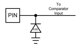
Figure 36: Analog Input Circuit
