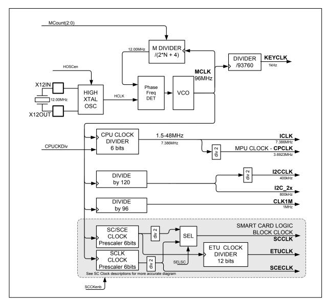
Figure 3: Clock Generation and Control Circuits
