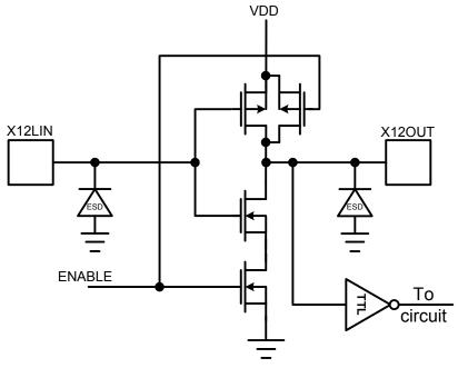
Figure 26: 12 MHz Oscillator Circuit
