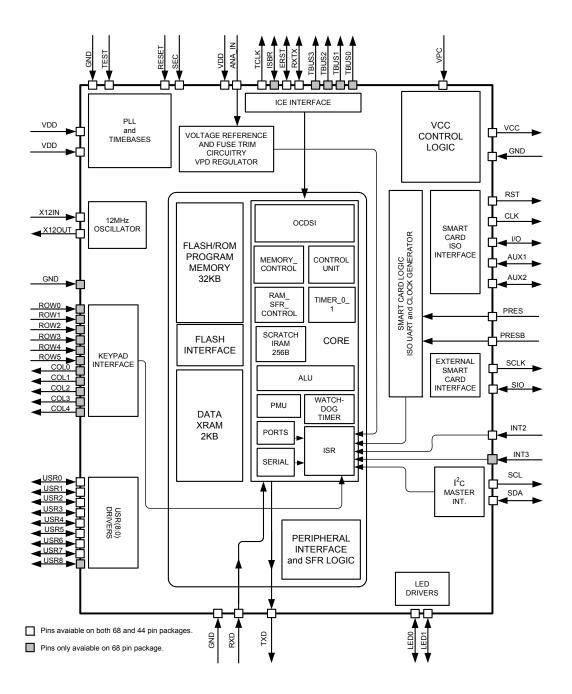
Figure 1: IC Functional Block Diagram
