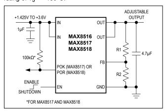
Figure 1. Typical Application Circuit
